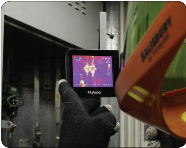
**Figure 14.** Infrared thermal scan.
