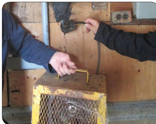
**Figure 11.** Fire started at box heater with receptacle and plug.
